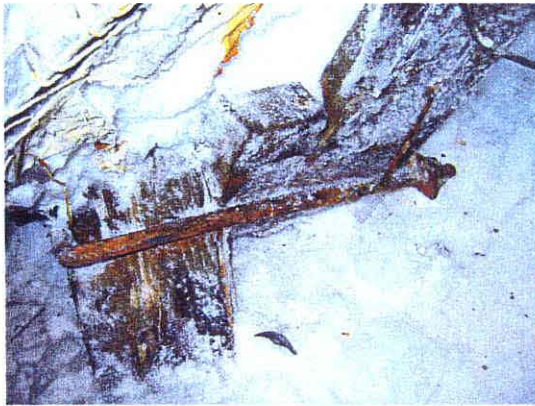
'U' BOLTS STILL FIXED TO BROKEN COLLAR TIES IN THE ICE
