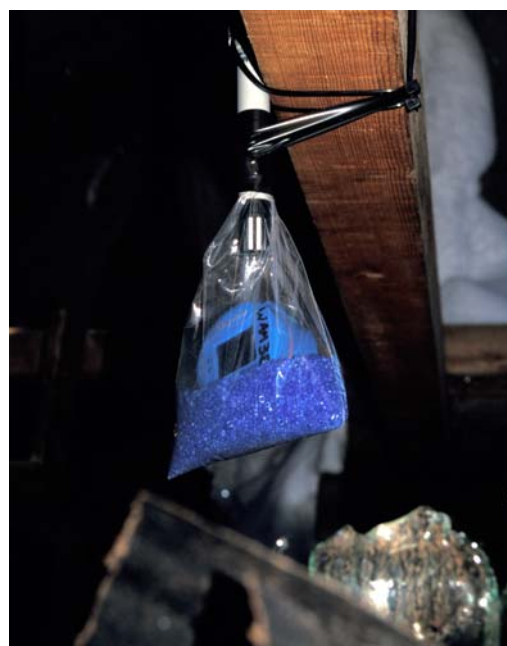
Drying and calibration check of Vaisala sensor
