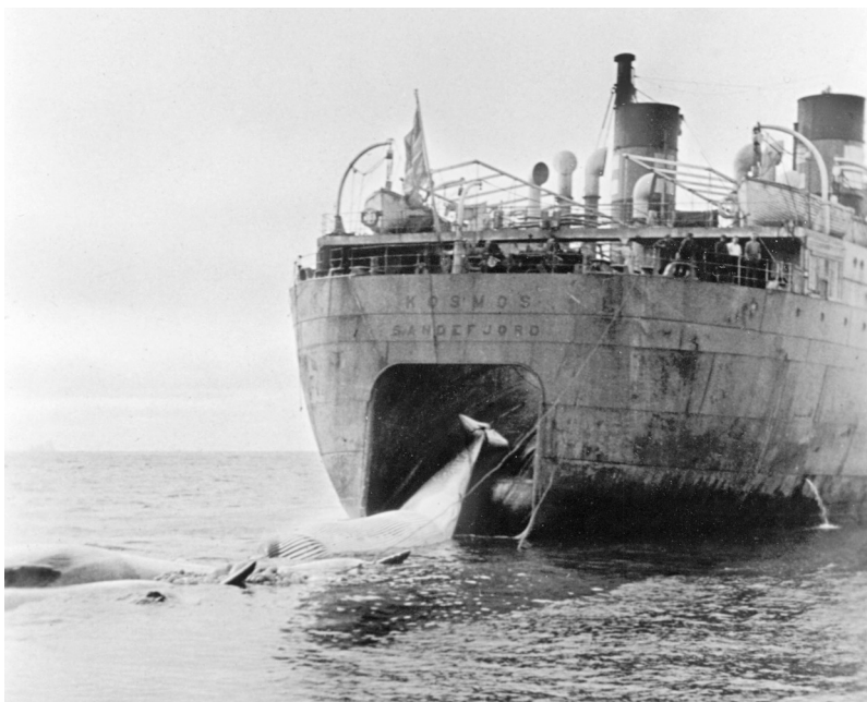
Plate 21. A whale being drawn up the stern ramp of the whale factory ship 'Kosmos' (BANZARE, Photo: E. Bond)
