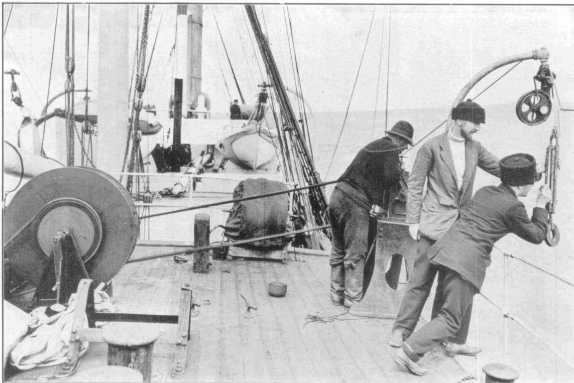
FIG. 3.—READING THE TEMPERATURE RECORDED ON ARRIVAL OF THE EKMAN REVERSING WATER-BOTTLE AT THE SURFACE.
