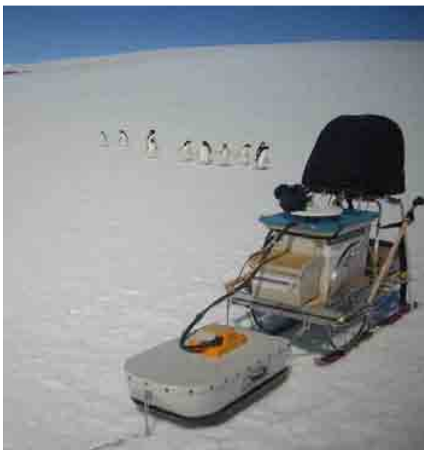
Figure 52: Ski attachments make the cart much easier to push on a rough surface. Penguins found the whole exercise fascinating.
