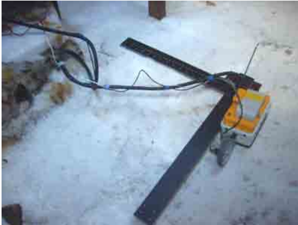
Figure 42: The equipment ready to scan an area of about 0.8m square near the table. The 800Mhz aerial and trigger wheel is run along the guide bar. The guide bar is moved along the fixed bar which is screwed to the ice (the bar is shown top left with registration holes). The guide bar (T piece) is held in place by the tent peg.
