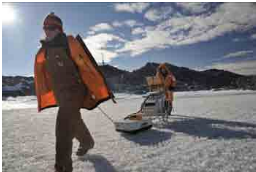
Figure 51: Surveying Round Lake. Note very rough ice surface. The process was much improved by using the ski attachments to the cart. (Photo David London)
