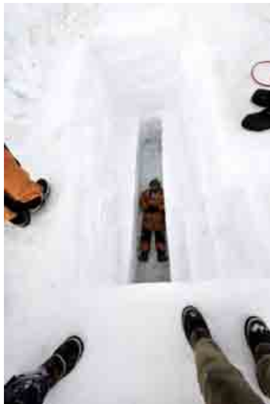
Figure 23: start of second dig. The coats hang on the post at the centre of the circular search area. The small orange tag in front of the chainsaw (arrow) is the spot where the three transit lines cross and represents the position where the air tractor frame was until its last sighting in 1976. (Photo: David London)
