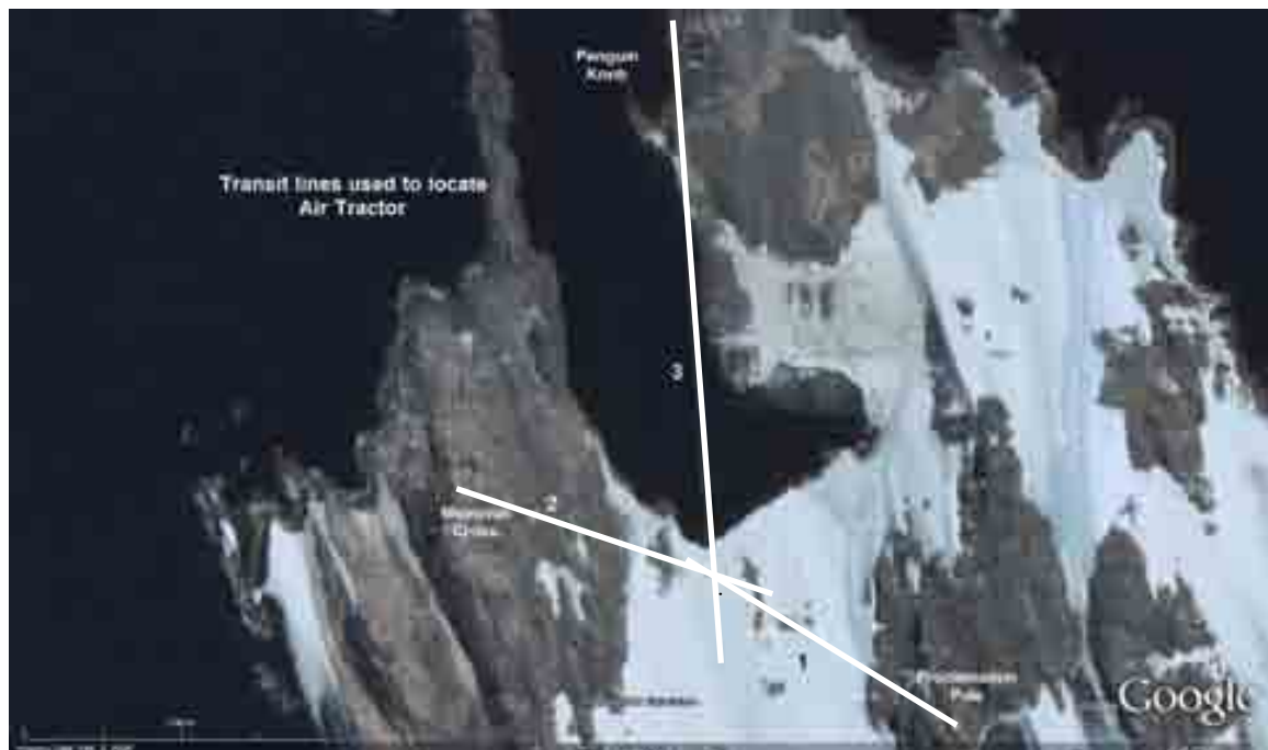
Figure 7 : Google earth picture of Cape Denison showing the three transit lines (white)) derived from a study of images from 1931 and 1976. The lines were used to pinpoint the position of the air tractor frame.
