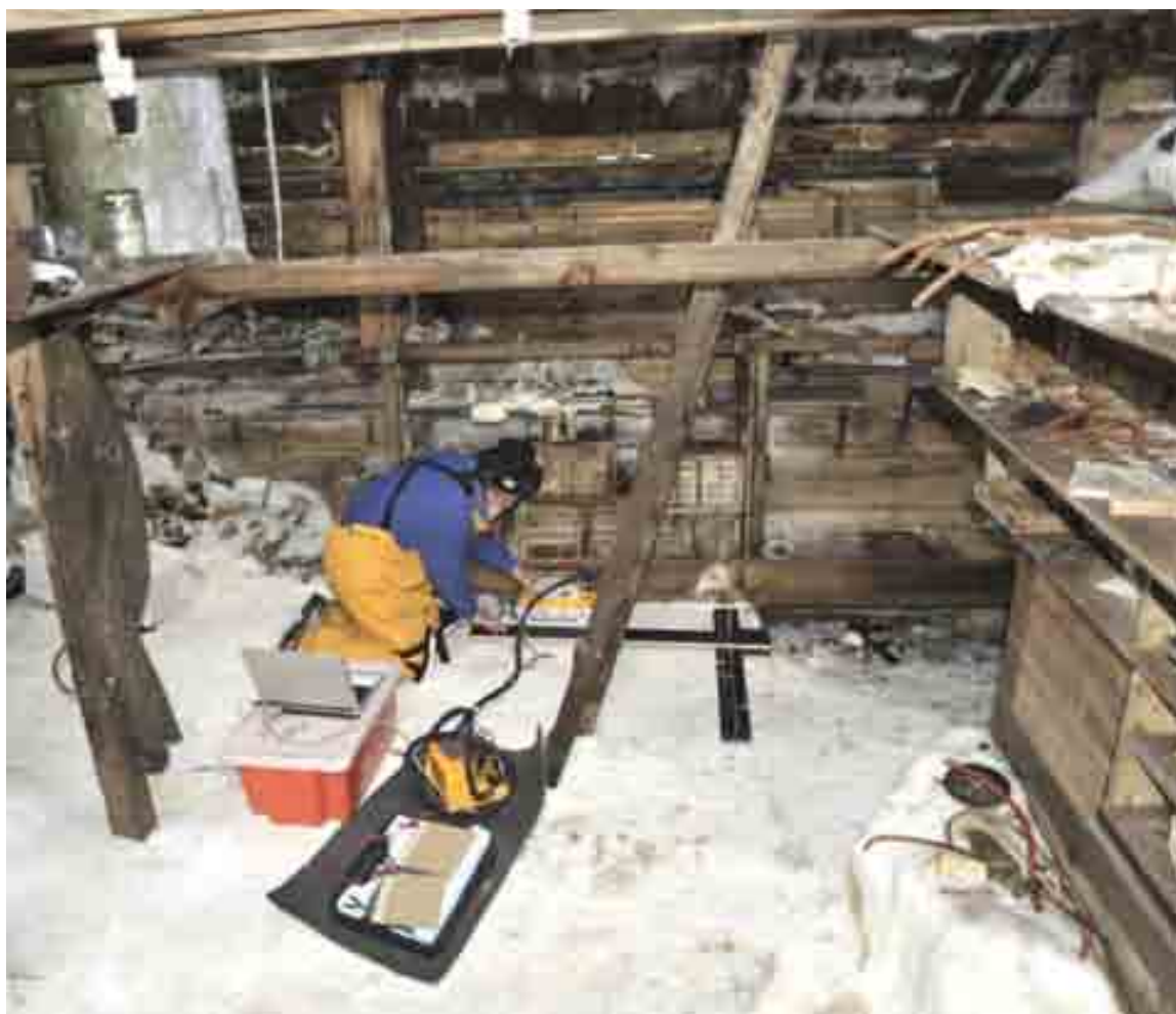
Figure 43: Scanning next to the bunk of J. H. Close. The floor was undulating but relatively smooth. Four areas were chosen where the guide bars allowed easy movement of the aerial. (Photo David London)
