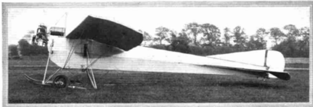
The Vickers Monoplane.—Side view, showing the protruding engine and the manner in which the wing trusses are carried to the base of the fuselage. An idea of the wing cross section may also be gathered.
