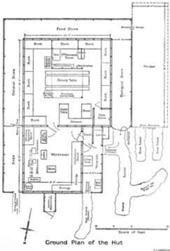
There is no direct external access. Entry is via the workshop, which is attached to the northern side of the living section. The rectangular workshop, prefabricated by Messrs Anthony (Melbourne), 5.5 m by 4.9 m, has a hipped roof and two skylights. The western verandah contains access to the cellar and roof as well as a latrine.
